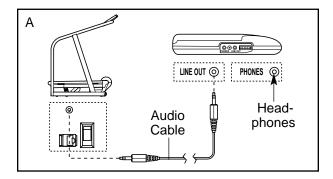
B. Plug one end of the audio cable into the jack on the side of the trainer near the power cord. Plug the other end of the cable into a 3.5mm Y-adapter (available at electronics stores). Plug the Y-adapter into the PHONES jack on your CD player. Plug your headphones into the other side of the Y-adapter.
